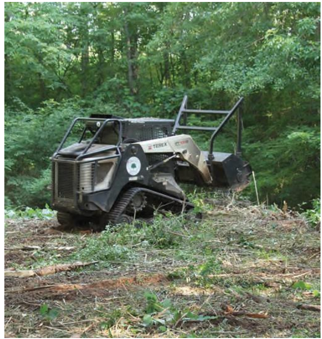
Figure 3. Skid steer mulchers can quickly grind dense stands of privet to the ground.
