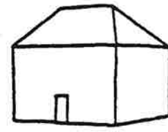
HIPPED ROOF WITHOUT FULL-WIDTH PORCH
