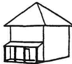
HIPPED ROOF WITH FULL-WIDTH PORCH
