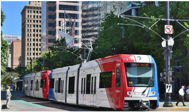
Catenary poles and wiring should incorporate street lighting and be aesthetically appealing
