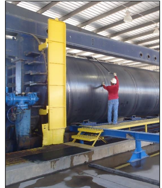
Hydraulic pressure testing of pipe at factory
