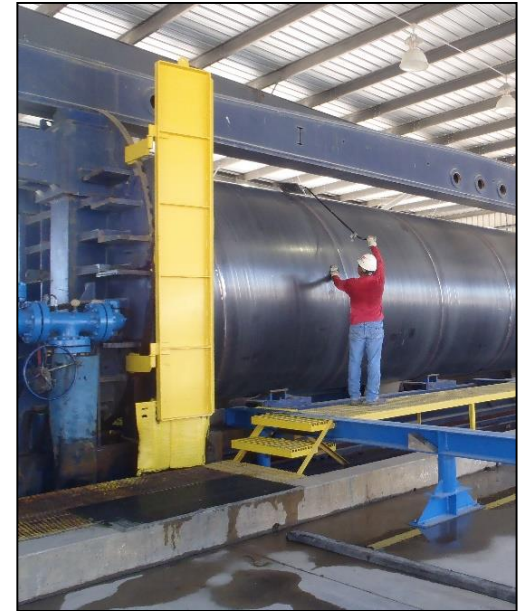
Hydraulic pressure testing of pipe at factory
