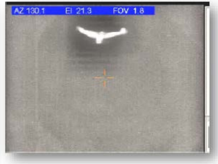
Thermal imaging detector close-up of hawk at 15x zoom at a range of approximately 4.5 miles
