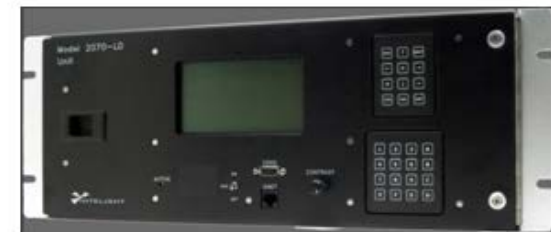
Traffic Signal Controller
