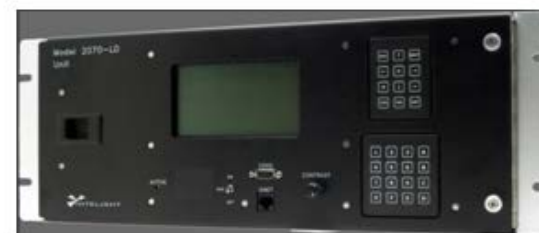
Traffic Signal Controller
