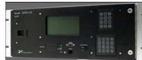
Traffic Signal Controller
