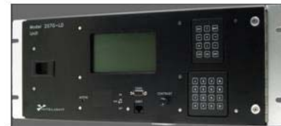
Traffic Signal Controller
