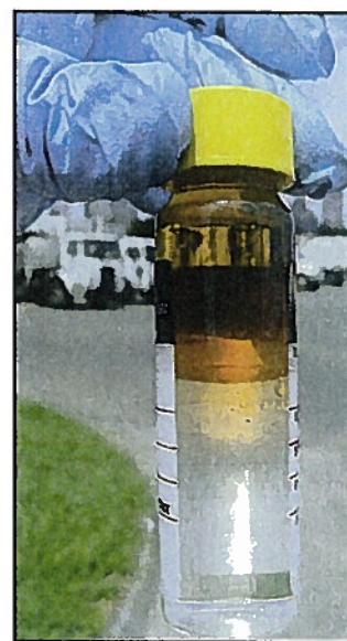
Figure 1: Weathered gasoline LNAPL floating on top of a groundwater sample.
