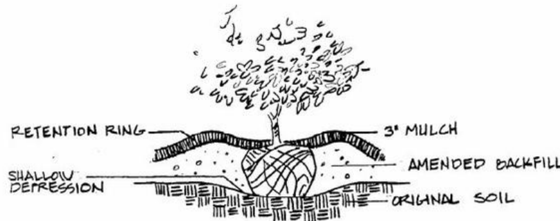
Figure 1. Shrub planting Illustration provided by NC State Extension, Planting Techniques for Trees and Shrubs Author, Kim Powell, Spec (Commercial Landscaping), Horticultural Science
