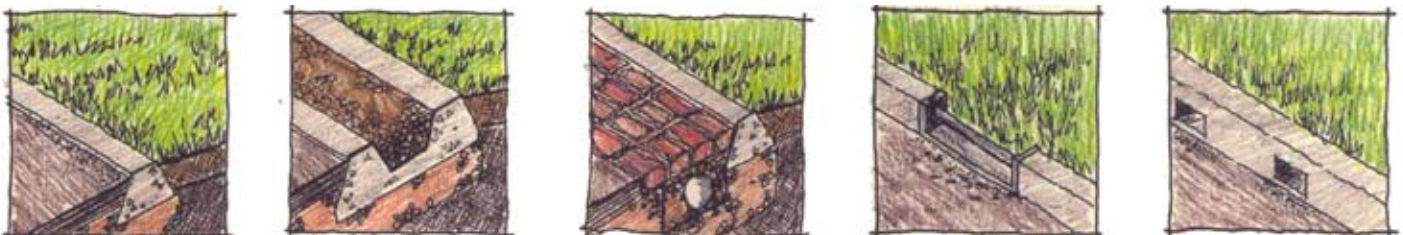
Examples of curb cuts that take pressure off the municipal storm water drainage system by allowing on-site filtration. Source: Portland Metro Green Streets Manual
