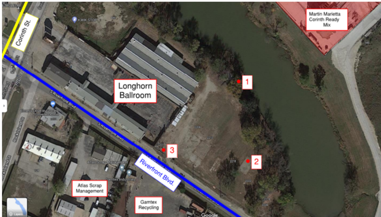
Satellite image indicating project site, measurement locations and notable noise sources.
